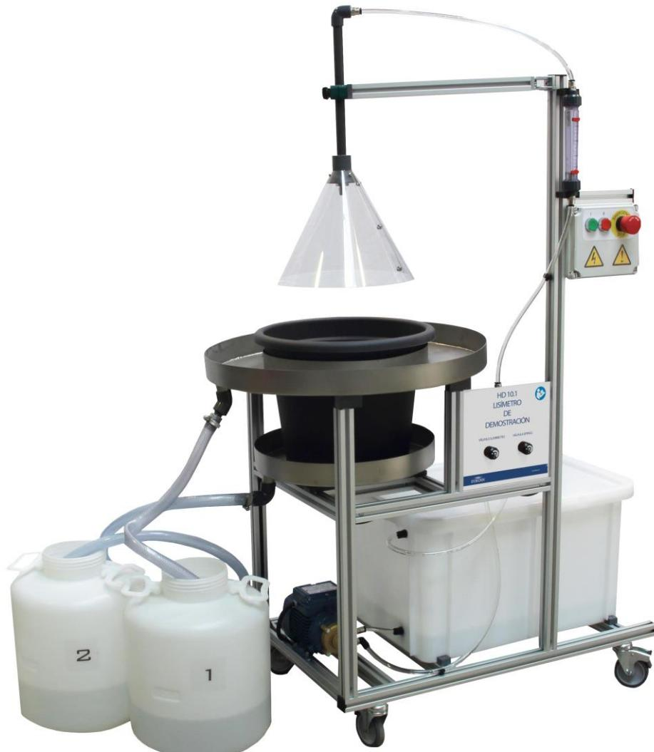
With the HD 10.1 equipment, it is a question of knowing the water retention capacity of a soil using the hydrological balance, differentiating each one of its elements.
